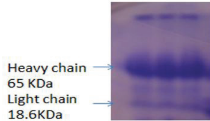
Figure 1: SDS – PAGE of chicken IgY. Heavy and light chains of IgY were distinctly separated as indicated by arrows; 10µl of IgY solution (0.5µg/µl) was loaded per well and SDS – PAGE run under reducing conditions.
